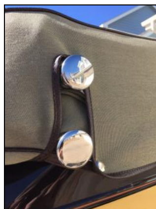
Folding landau iron shown in under-center unlocked position.
