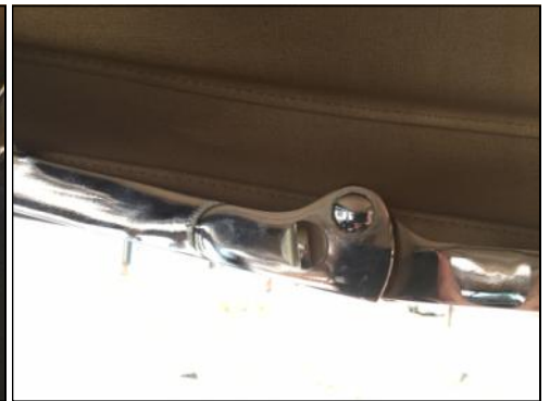
Folding irons over the side windows are released out of rigid position by operating the lock mechanism.
