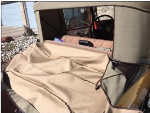
The boot cover snaps on, inside out, before the top is lowered.
