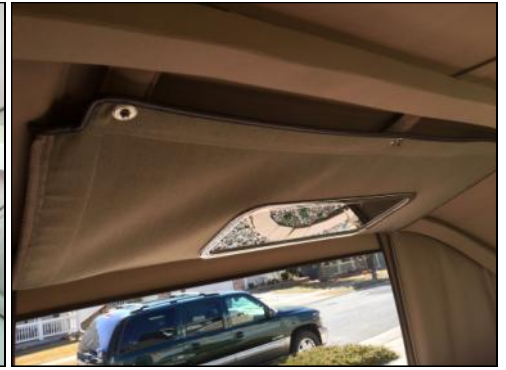
Back panel is snapped into position on the attach points between #1 and #2 roof bows.
