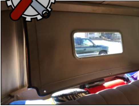
Cloth back panel with rear window is unzipped, unsnapped, and pushed inside of car.
