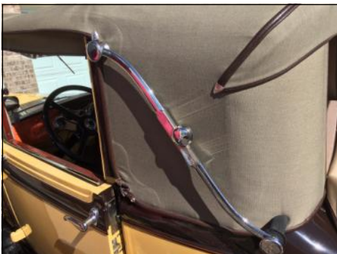
Folding landau iron shown in over-center locked position.
