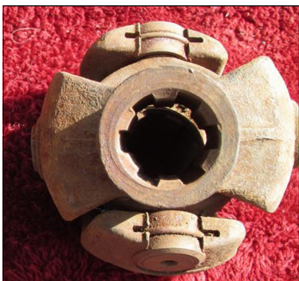
This is an original non-riveted u-joint
