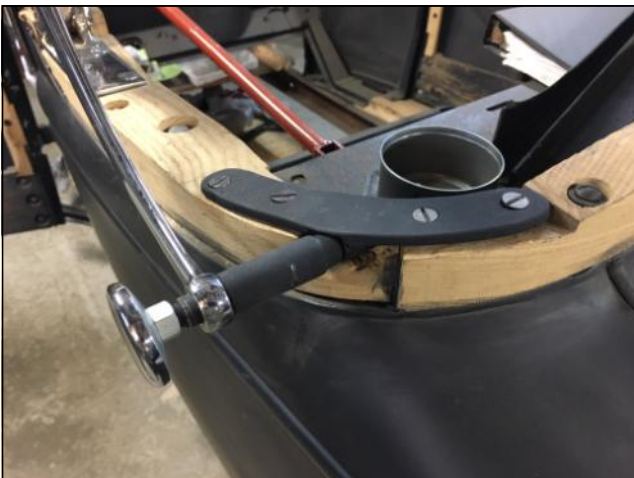
Custom lower landau bracket, with post that threads into bracket.
