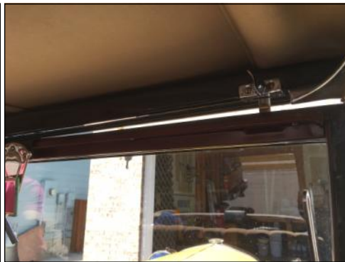
Wing nut screws are unscrewed to allow the beader to come up and off of the windshield frame posts.
