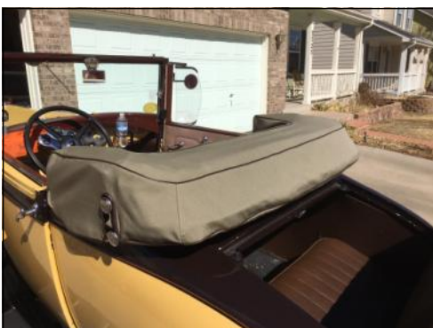
Boot cover wrapped up and over lowered top...
