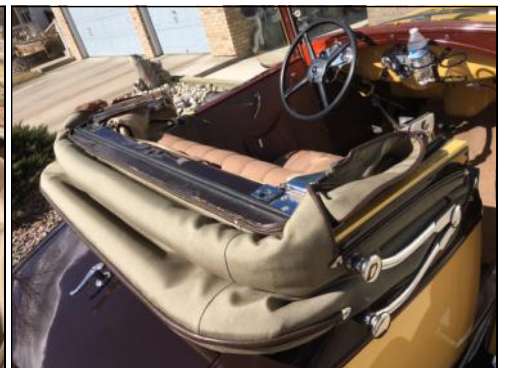
Top is folded down, making sure the cloth top material folds inwards.
